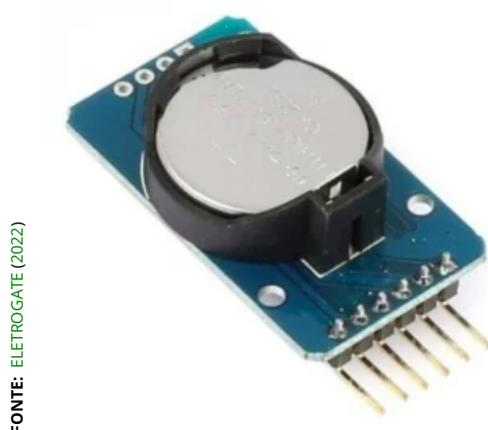
**Figura 3.10** – Módulo RTC.
